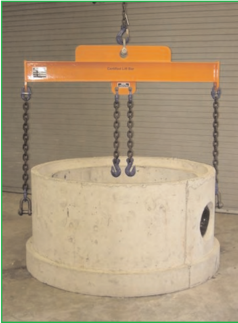
Certified A-LOK lift bar with Choker chains for lifting cones.
